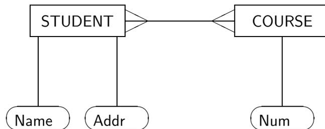
The information in such a diagram can be represented by a directed graph in the following way. The first step is to replace a line representing a relationship by a new entity and (e. g. in the case of a binary relationship, two) directed edges (arrows) to the entities related. Thus we represent the relationships by *tabulating spans*. This places entities and relationships on the same level (represented by boxes) with arrows among them. Then
