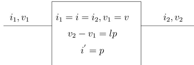
Using the operations of  $\mathbf{TSpan}_{\mathbb{R}, \mathbb{R}}(\mathbf{Graph})$  one can now evaluate a network of resistors, capacitors and inductors. For example the circuit of an inductance and a capacitance
