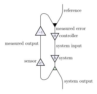
The user inputs a 'reference' signal, which is fed into a controller, whose output is fed into a system, or 'plant', which in turn produces its own output. But then the system's output is duplicated, and one copy is fed into a sensor, whose output is added (or if we prefer, subtracted) from the reference signal.
