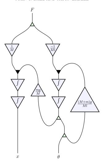
As a start, one can use Theorem 4.2 to prove that it is indeed possible to do this rewriting. To do this, simply check that both signal-flow diagrams define the same linear relation. The proof of the theorem gives a method to actually do the rewriting—but not necessarily the fastest method.
