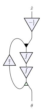
Note that this already includes a kind of feedback loop, since the pendulum's angle affects the force on the pendulum.
