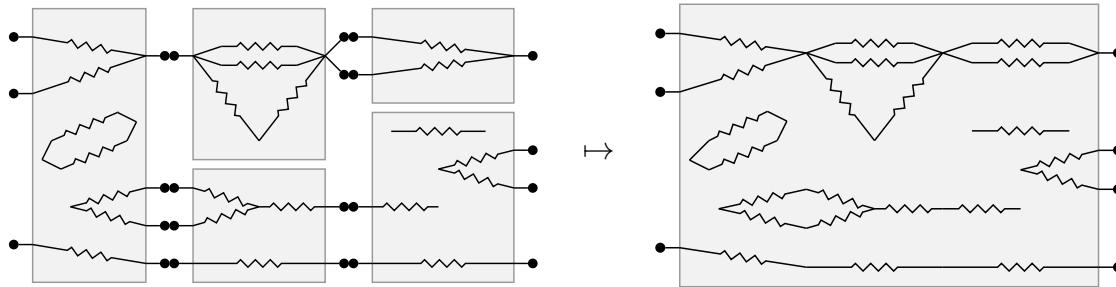
Note in particular that the composite of these circuits contains a unique resistor for every resistor in the factors. If we are interested in describing the syntax of a diagrammatic language, then this is useful: composition builds given expressions into a larger one. If we are only interested in the semantics—given, say by the electrical behaviour at the terminals—this is often unnecessary and thus often wildly inefficient.
