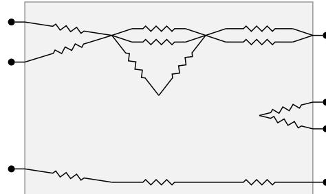
where we have removed circuitry not connected to the terminals. Moreover, this second circuit is a more efficient representation, as it does not model inaccessible, internal structure. If we wish to construct a category modelling the semantics of open circuits then, we require circuit representations and a composition rule that only retain the information relevant to the black boxed circuit. In this paper we introduce the notion of corelation to play this role.
