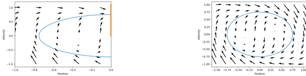
(a) The continuous mode of H_{\text{hop}} with its guard Z_v in orange and its attracting limit cycle g(S) in blue. The reset map reflects any point in the guard through the origin.
